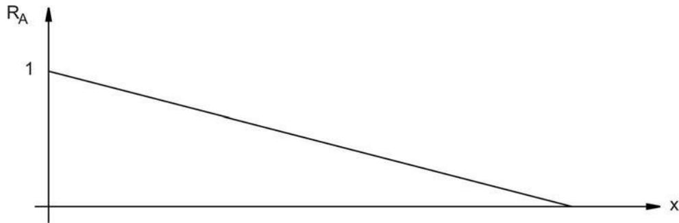
**Figure 7.3: Influence line for support reaction A**
