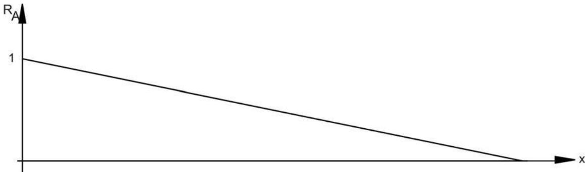
Figure 7.11: Influence line for support reaction at A
