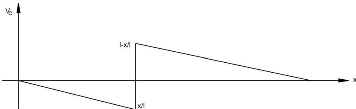
**Figure 7.13: Influence line for shear at section C**
