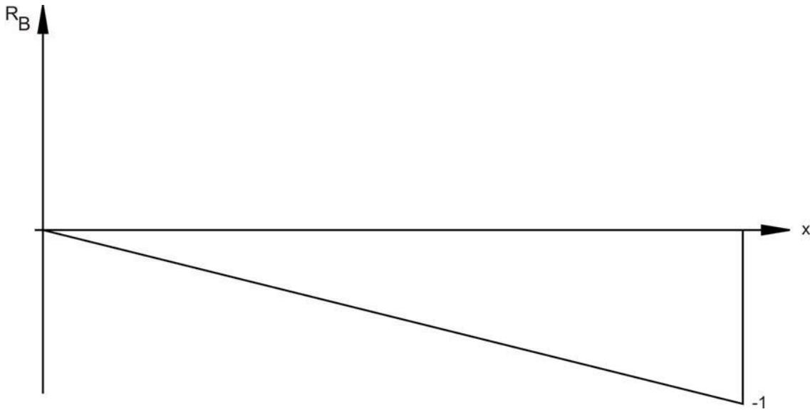
**Figure 7.12: Influence line for support reaction at B**
