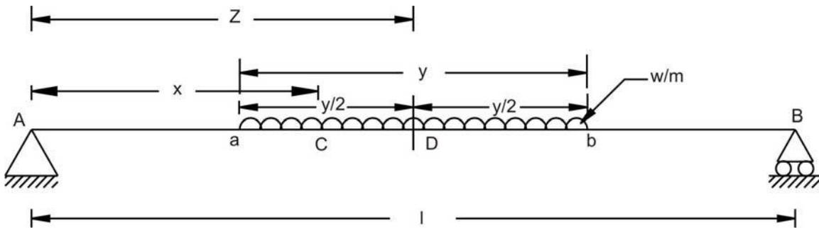
Figure 7.16: Beam loaded with UDL shorter in length than span
