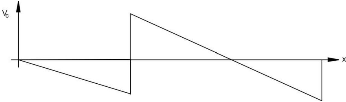
**Figure 7.6: Influence line for shear at section C**
